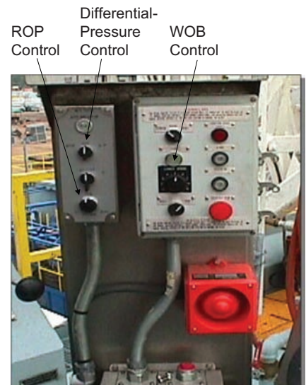
Fig. 1—Controls for electronic autodriller with proportional disk brakes.
