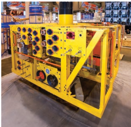
Fig. 3—GE Oil & Gas VetcoGray DHXT deepwater horizontal tree.
