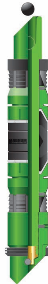
Fig. 2—Magnum Oil Tools International’s Rapid Mill composite fracturing plug.
