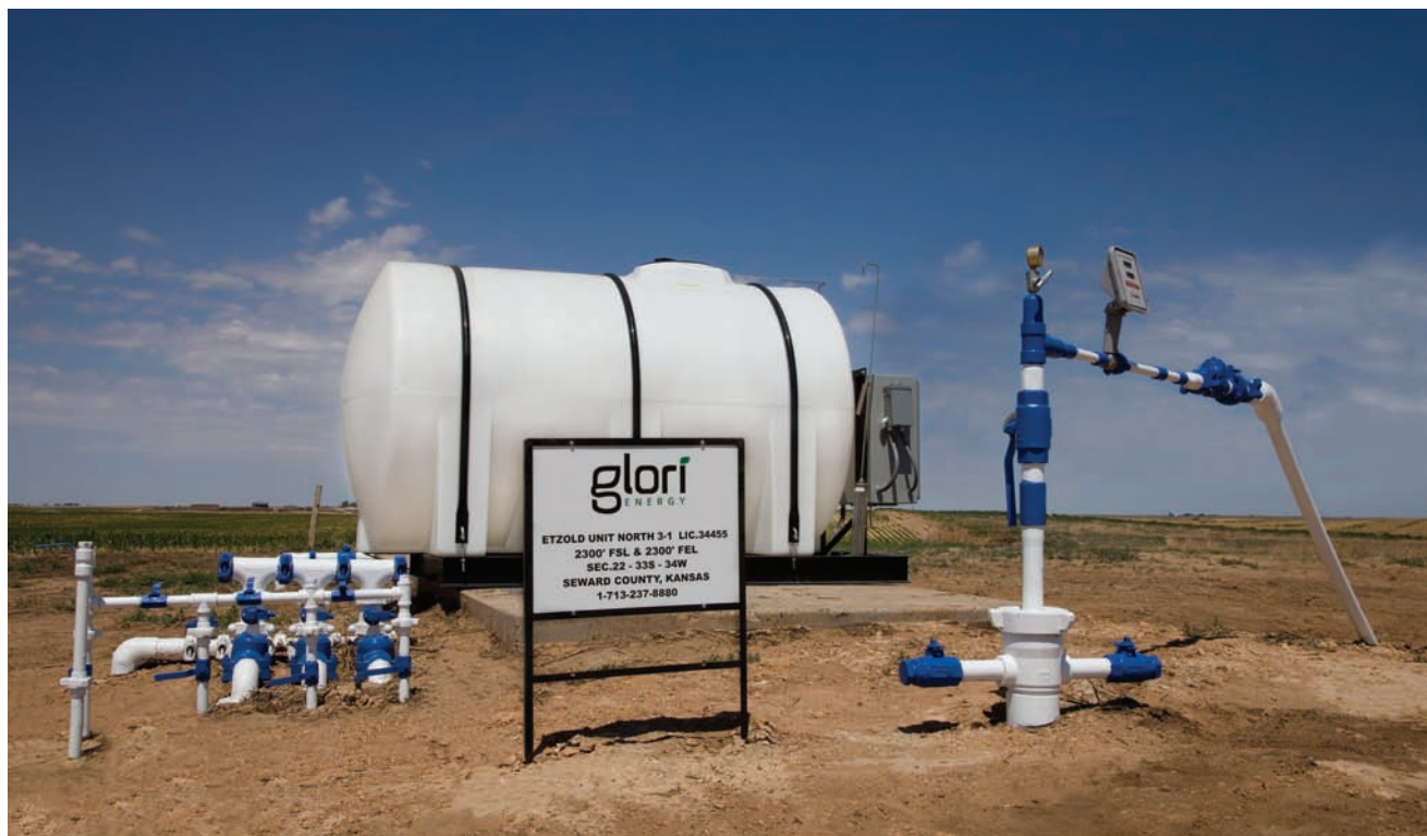
Tanks like this one are used by Glori Energy to pump its nutrient mix into an oil field. The blend is customized to encourage the growth of certain bacteria said to promote production in older fields.
