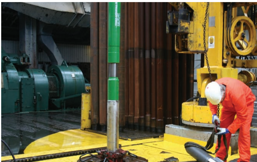
Fig. 1—The antistall tool must be placed within 50 m of the bit. Typically the tool goes on top of the nonmagnetic section or above the underreamer, where applicable. (Photo courtesy of Tomax.)
