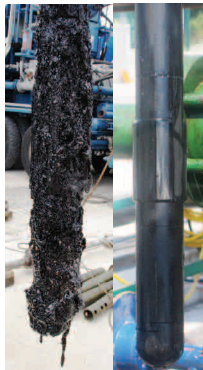
Fig. 4—Bottomhole assembly with asphaltene (left) and with Halliburton's DuraKleen service (right).
