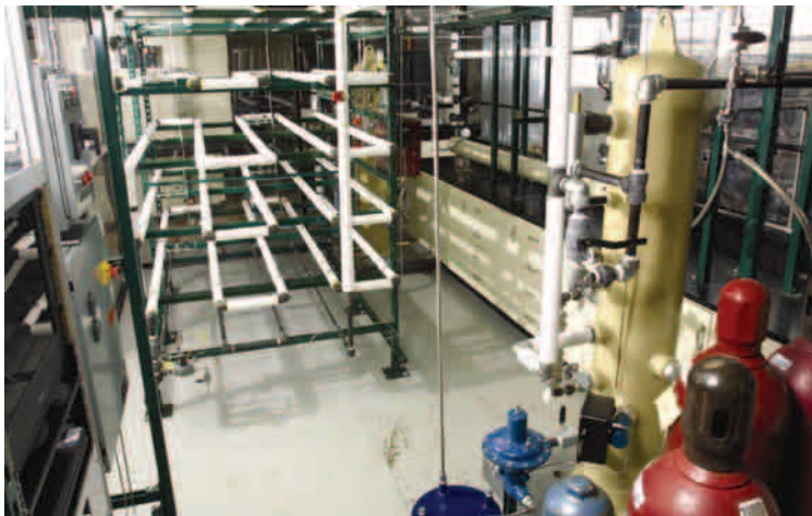
Fig. 1—A schematic and photograph of the scavenger test loop at the Gas Technology Institute are shown.
