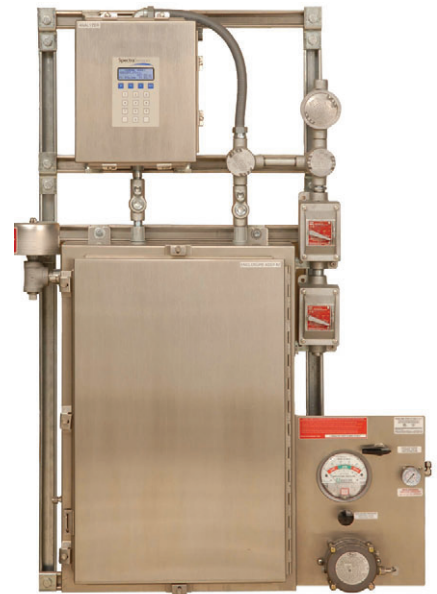
Fig. 4—The SpectraSensors system comprises a sample cell that the gas flows through, a tunable-diode laser that emits a specific wavelength of light through the gas, an optical detector, and software to analyze data and deliver the results.
