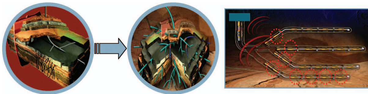
Fig. 2—MRC wells will give way to extreme-reservoir-contact wells. Right: Wireless telemetry will allow an unlimited number of smart laterals and an unlimited number of valves per lateral.
