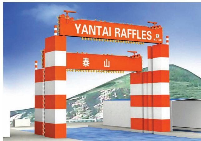
Fig. 5—The Taisun gantry crane.
