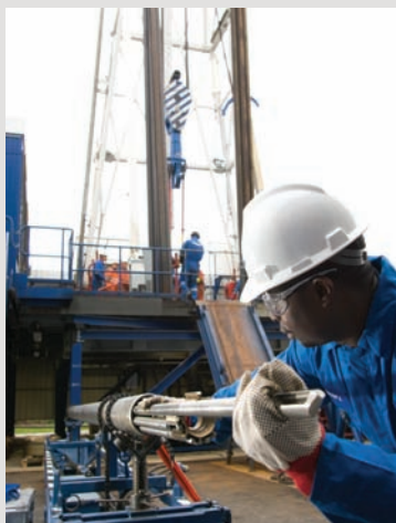
A Schlumberger specialist prepares a SCAR sample carrier to run slimline single-phase reservoir fluid samplers on a drillstem test.
