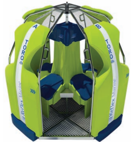
Fig. 7—Reflex Marine's TORO personnel-transfer capsule.
