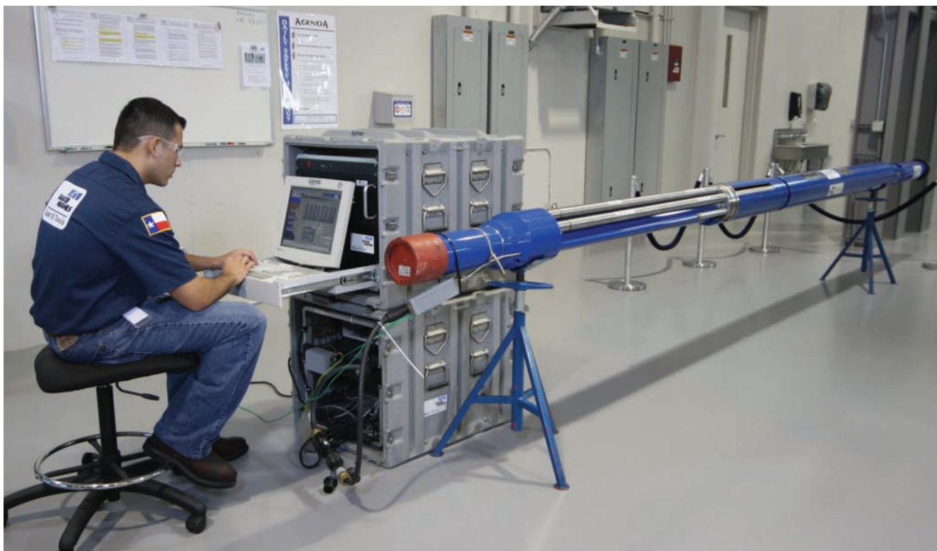
An engineer tests the functionality of downhole gauges on an Intelligent Well System at Baker Hughes’ Center for Technology Innovation in Houston.
