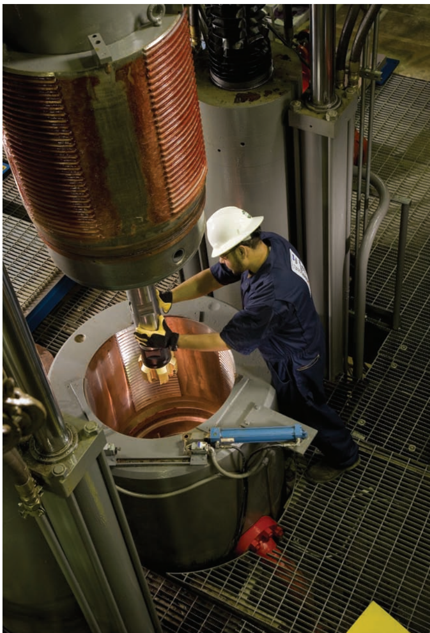
At Baker Hughes' drilling simulator lab in The Woodlands, Texas, this pressurized test simulator is used to reproduce downhole stresses on the rock while drilling.
