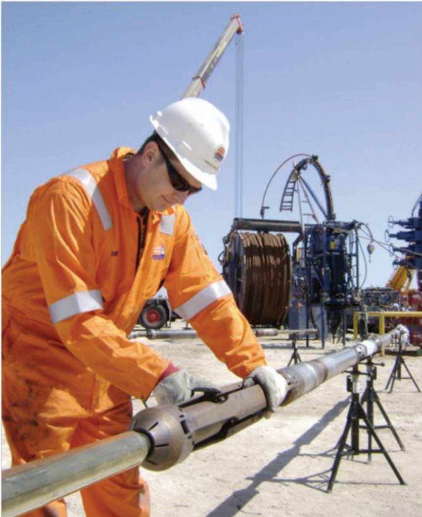
Fig. 3—Western Well Tool’s IT-470 Tractor for use with CT.
