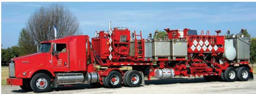
Fig. 3—Halliburton’s trailer-mounted AOF blending system.
