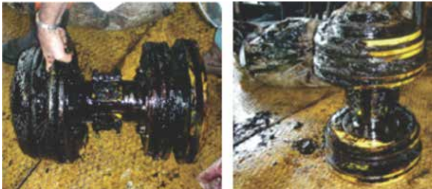
Fig. 19—Wax/oily deposits returned by means of the Bi-Dis post-sand removal.
