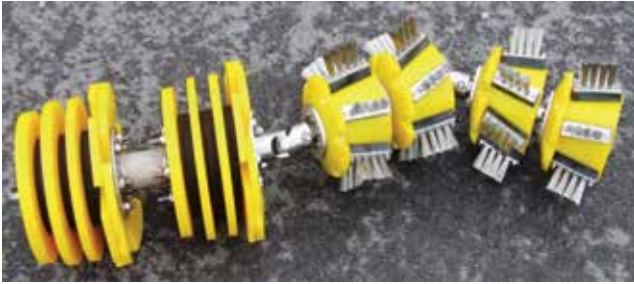
Fig. 7—Articulated pig; front-sealing module followed by brush modules at rear.
