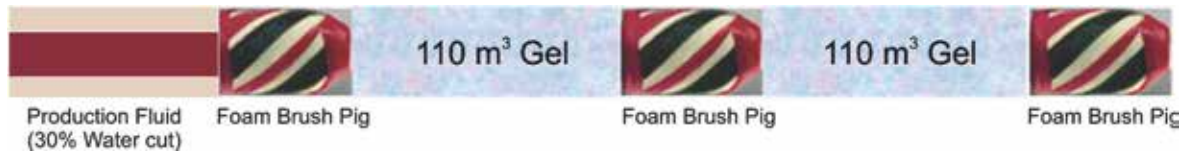
Fig. 21—Once-through sand removal gel train.
