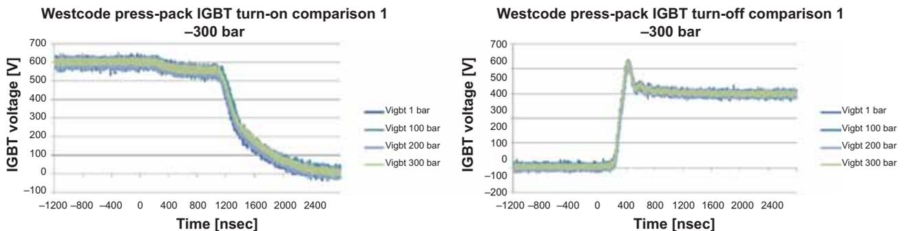
Fig. 9—IGBT turn-on and turn-off voltage waveforms at different pressures between 1 and 300 bar.
