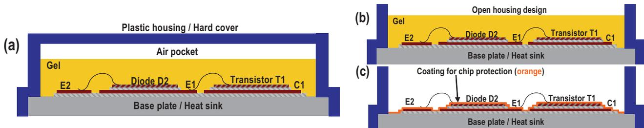
Fig. 2—(a) Common structure of planar IGBT with internal air pocket, (b) concepts for adaptation to pressure tolerance with open IGBT housing with original gel, and (c) with special coating layer for protection of power semiconductor chips.
