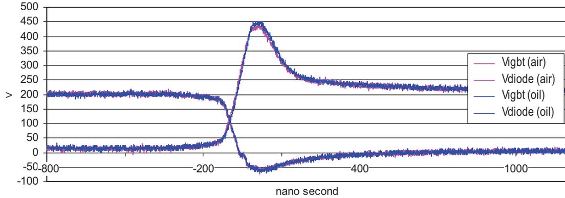
Fig. 5—Measurements of switching waveforms in air and in dielectric liquid (Midel®7131) at 1 bar.
