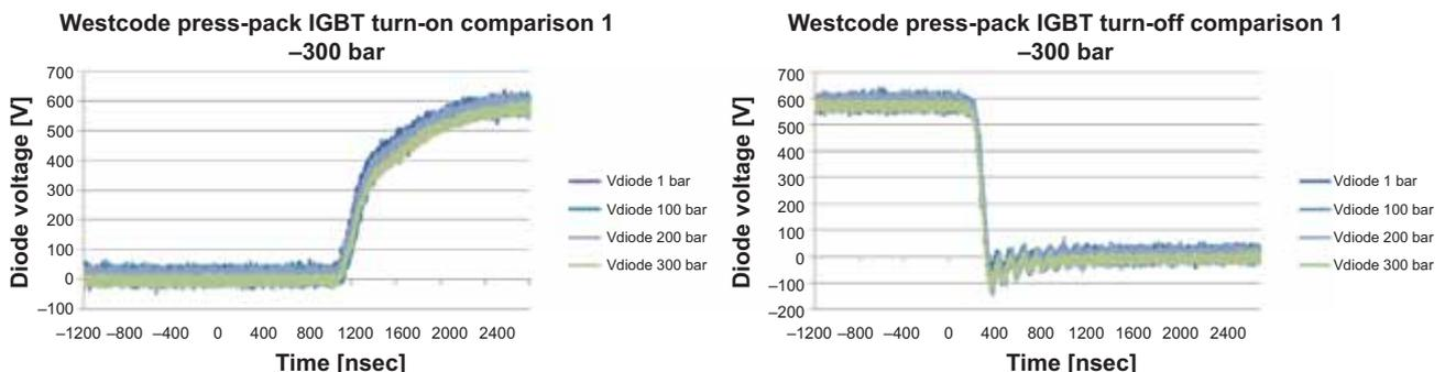
Fig. 10—FWD voltage waveforms at different pressures between 1 and 300 bar at IGBT turn-on/off.
