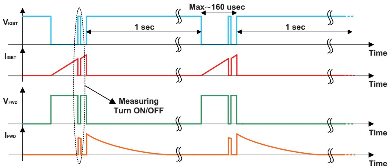
Fig. 3—Double-pulse-testing waveforms.
