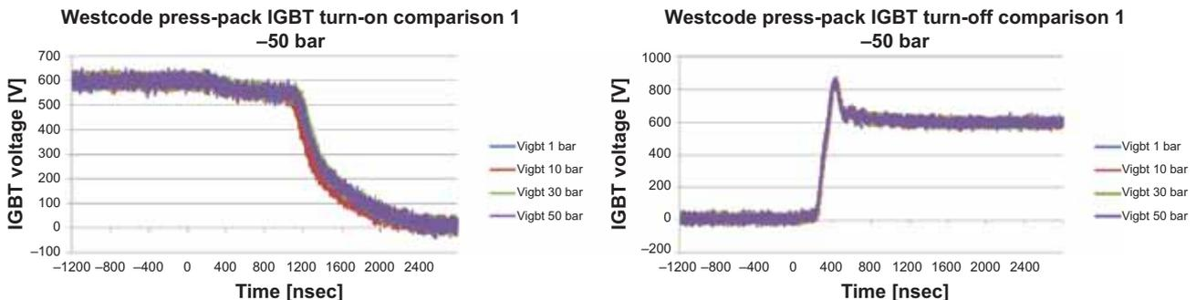
Fig. 7—IGBT turn-on and turn-off voltage waveforms at different pressures between 1 and 50 bar.
