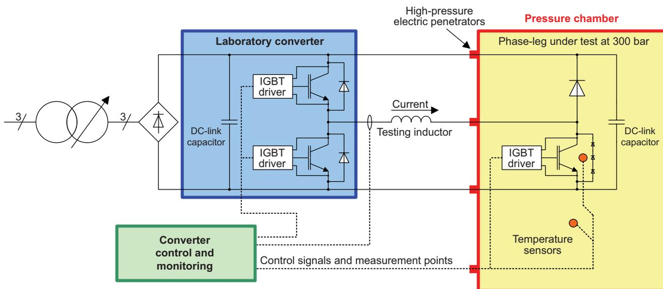
Fig. 4—Test-circuit diagram including the test object with devices under test (FWD and IGBT).
