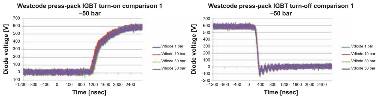
Fig. 8—FWD voltage waveforms at different pressures between 1 and 50 bar at IGBT turn-on/off.
