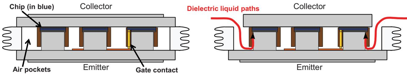
Fig. 1—Structure of an off-the-shelf press-pack IGBT (left) and concept for adaptation to pressure tolerance (right).
