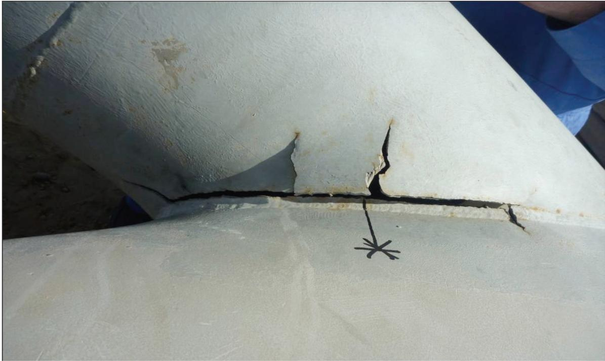
**Fig. 1—20-in.×16-in. flare header unreinforced branch after failure.**
