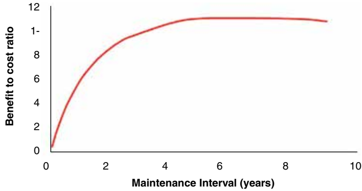
Fig. 3—Maintenance optimization of pipeline under structural defect.
