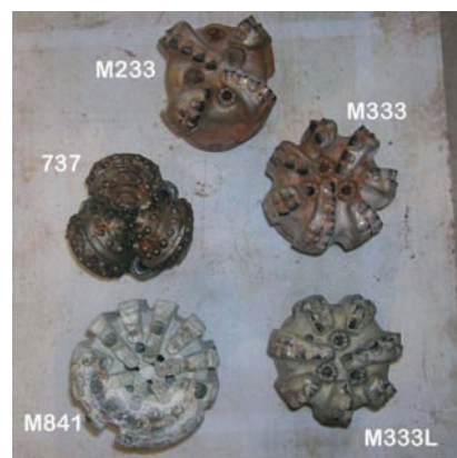
Fig. 1—Drill bits used in Phase-2 testing.
