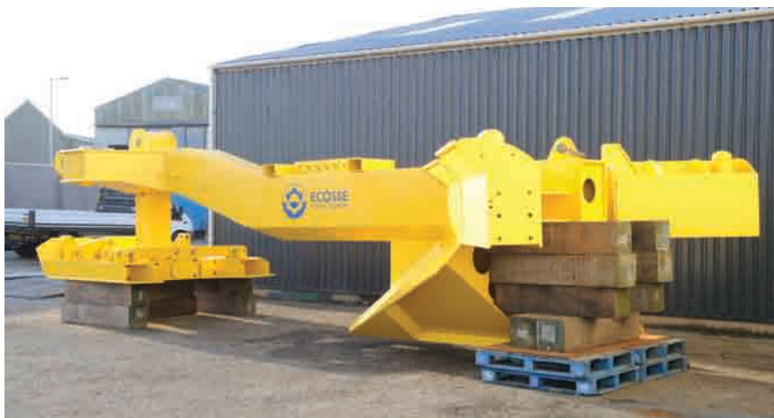
Fig. 4—Ecosse Subsea Systems' SCAR trenching plow.
