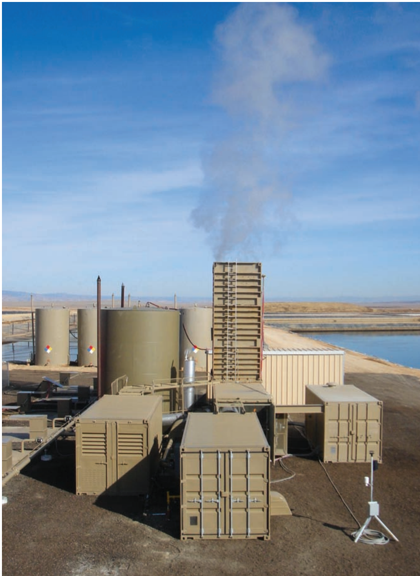
Using vapor recompression technology, Purestream's Trilogy unit reduces the cost of recycling fracturing water by using waste heat. The unit produces water vapor and solid residue that is disposed of in a waste facility.
